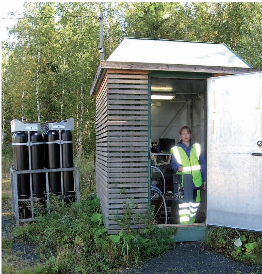
Water sampling from a deep borehole.
