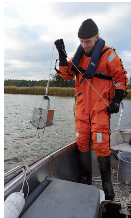
The seabed fauna studies forming part of the monitoring programme of the power plants were supplemented by Posiva's own sampling campaign in the autumn. The picture shows sampling in progress using an Ekman sampling device.
