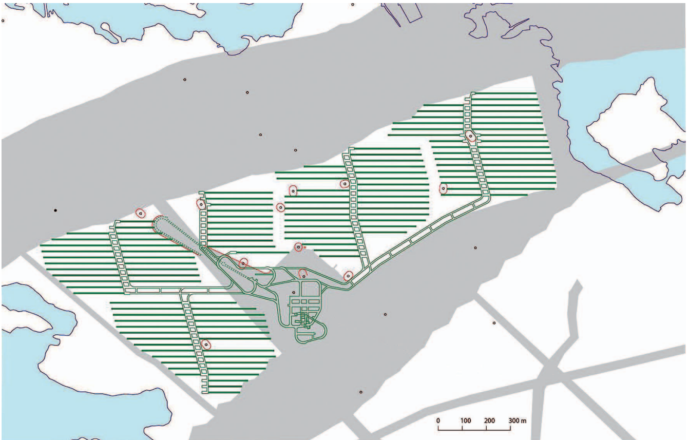
Layout alternative with the orientation of deposition drifts at 90/270 degrees.
