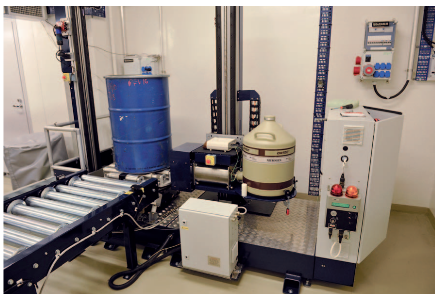
Gamma-spectroscopic measuring equipment for drum waste undergoing trial operation (determination of gamma activity, automatic drum conveyor, weighing rotator, etc.). Photo: Ari Haimi.
